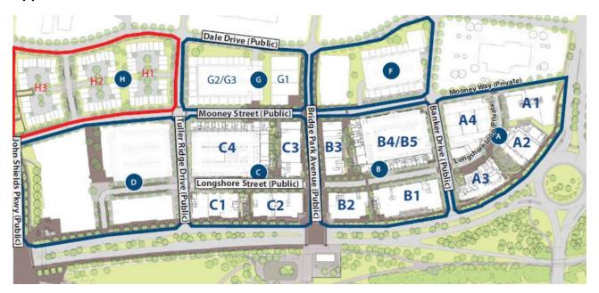
This is a request for review and informal, non-binding feedback for the construction of townhome units in Block H of Bridge Park. The project proposes 6 Single-Family Attached residential buildings. The buildings include ground floor parking access through an interior auto court with multi-level units surrounding. A new public street is proposed to connect Mooney Street to Dale Drive.
