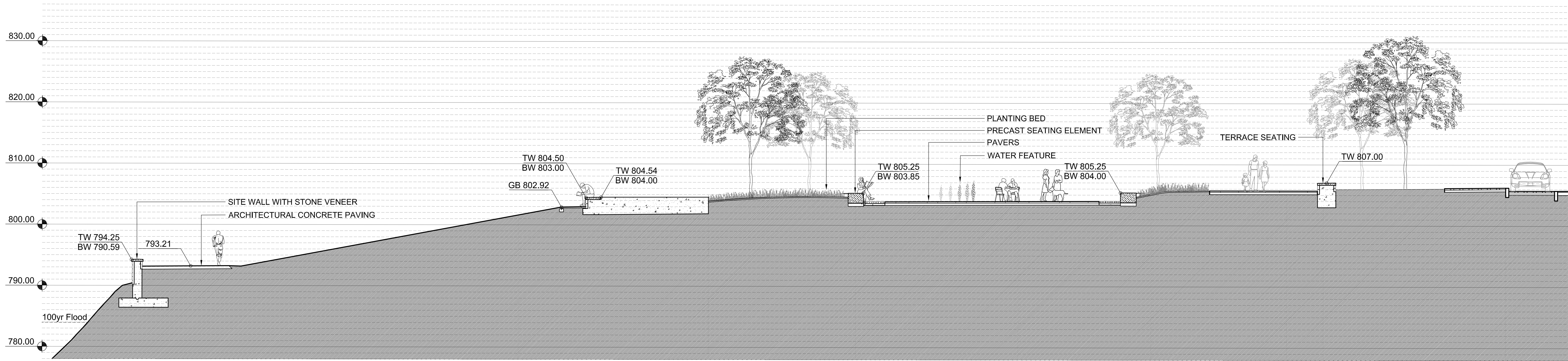
1 East Landing Section Through Lower Terrace
