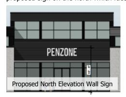
foot internally illuminated sign with individual white channel letters and black returns at a height of 16'6" from grade to the top of the sign. As proposed this sign meets the BSD Code requirements which permits a 50-square-foot sign located within the first story of the building.
