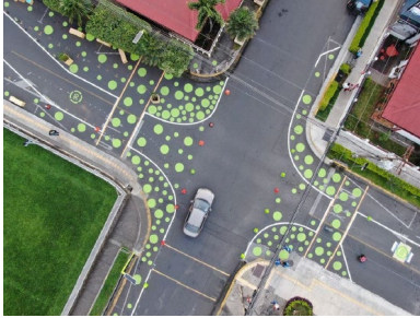
Curb Extensions Costa Rica
