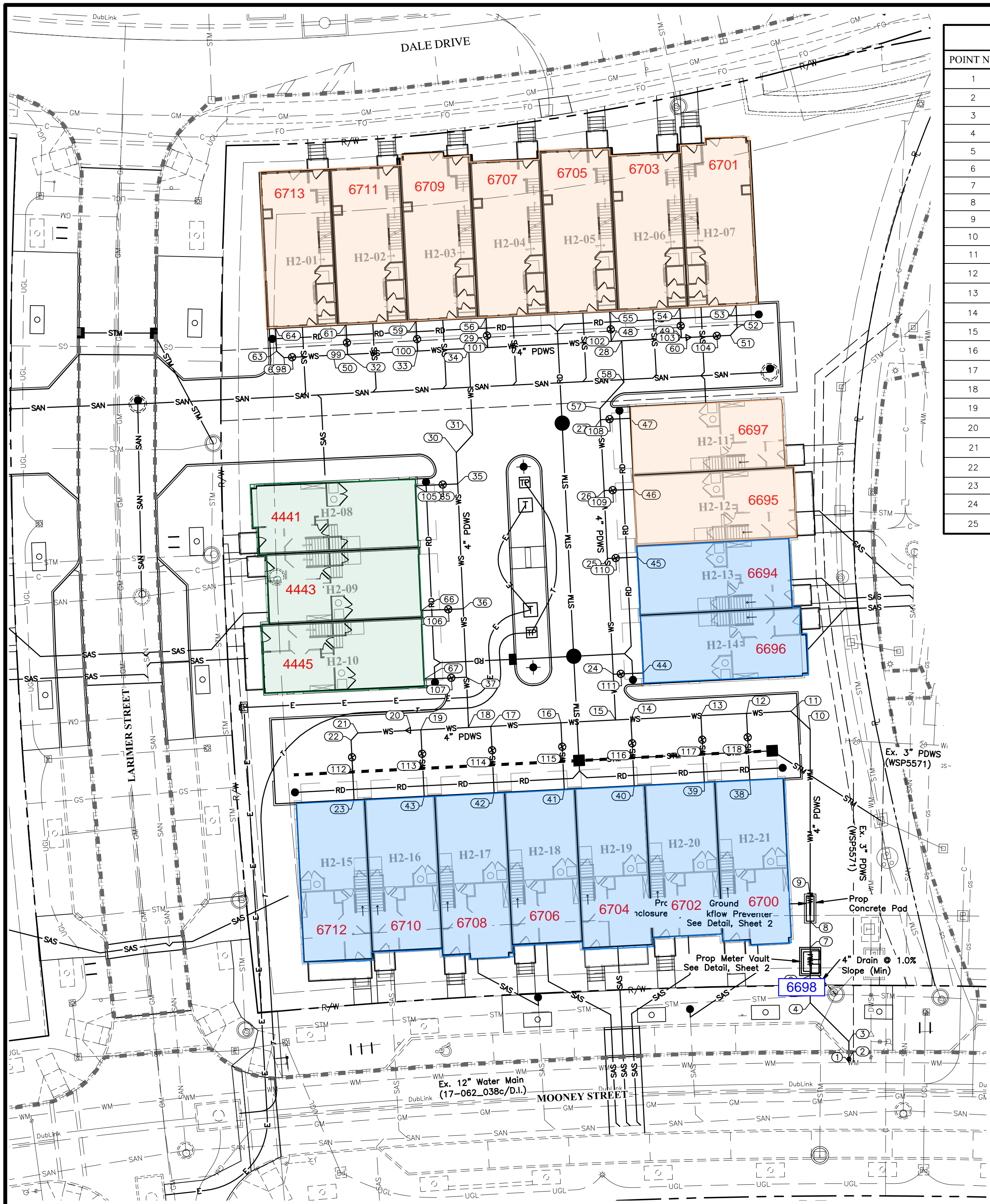
BLOCK H2 - WATER SERVICE PLAN Scale: 1" = 20'
