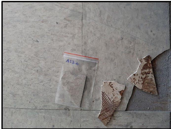
3 – HA 3 - Vinyl Floor Tile (White with Gray Mottles, 12"x12") with Mastic (Tan)
