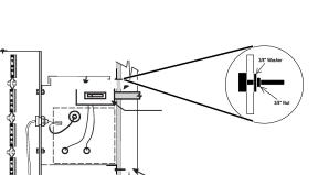
10- 3/8"x3" thru bolts attaching raceway to existing cabinet (5 attachments on top, 5 on bottom)
