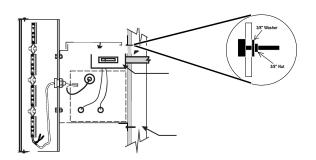
10- 3/8"x3" thru bolts attaching raceway to existing cabinet (5 attachments on top, 5 on bottom)
