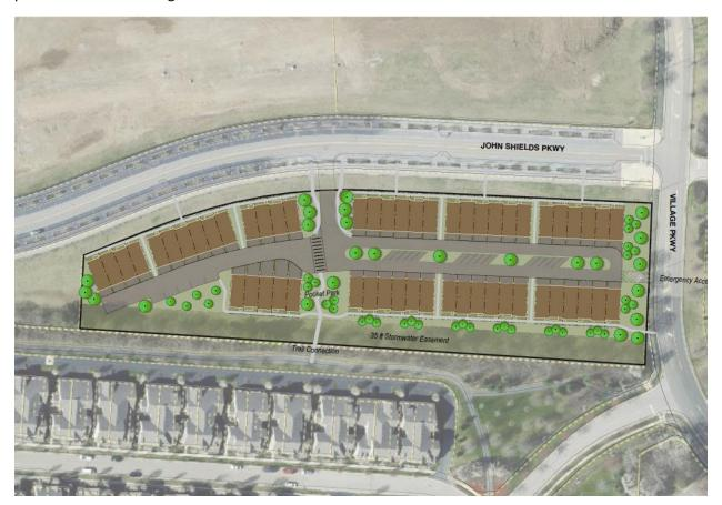
The site will be accessed primarily from a full movement intersection at John Sheilds Parkway and an emergency access along Village Parkway. The internal vehicular access would be a modified alley that would be wide enough to accommodate utilities and any emergency access as well as curbed guest parking and a landscaped median.
