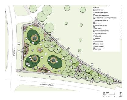
The proposed sidewalk along Dale Drive and north of the site will connect to the existing pedestrian network. The applicant proposes to create pockets of brick pavers along Tuller Ridge Drive, Dale Drive, and the sidewalk along Sycamore Ridge, along with seating. The applicant offers a 6' wide brick paver path throughout; however, it is reduced to approximately 4' in front of the benches. Staff recommends a continuous 6' wide brick paver path for a comfortable walking and sitting environment.
