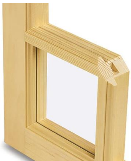
a) True Divided Light This type shows the traditional solid wood muntin wrapping a cut panel of glass. Note that there are no spacers as the glass is cut to fit inside the muntins. RECOMMENDED
