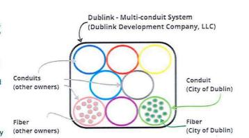
The outer black box represents Dublink's multi-conduit system. That system is owned by Dublink Development Company LLC and it consists of a number of different conduits within that they rent to other customers, including the City of Dublin. We own one conduit through which we run fiber. We own a number of different conduit and fiber outside of this bank system. The maps below attempt to illustrate these systems.
