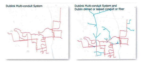
The map with only the red lines represents Dublink whereas the lines that are blue on the secondary map show more of the conduit with fiber inside of it that lies outside the Dublink system. Mr. Brown stated that we utilize a network topology called rings. What rings do is create redundancy, fast pathways and both high reliability and scalability.
