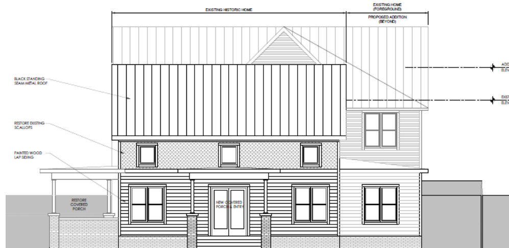
East Elevation: historic in darker line weight, addition in lighter weight behind
