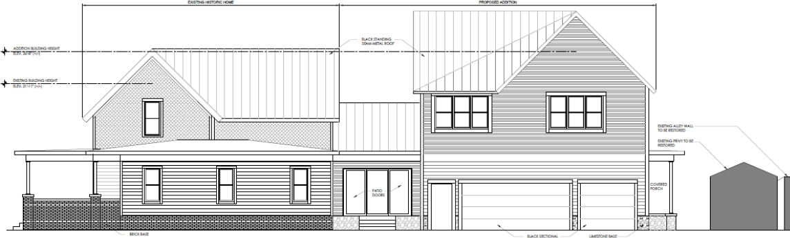
North Elevation: historic on left, addition on right with pyramidal roof form adjacent to hyphen
