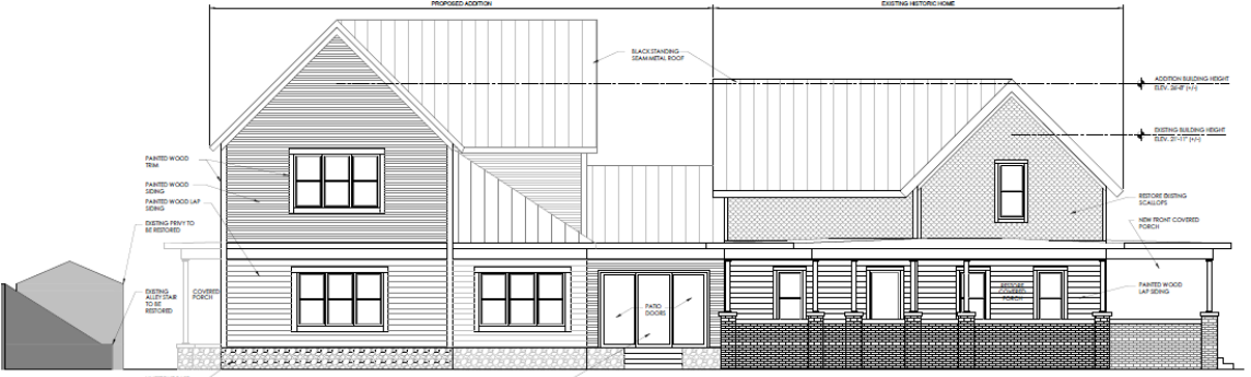
South Elevation: addition on left, pyramidal roof form adjacent to the hyphen
