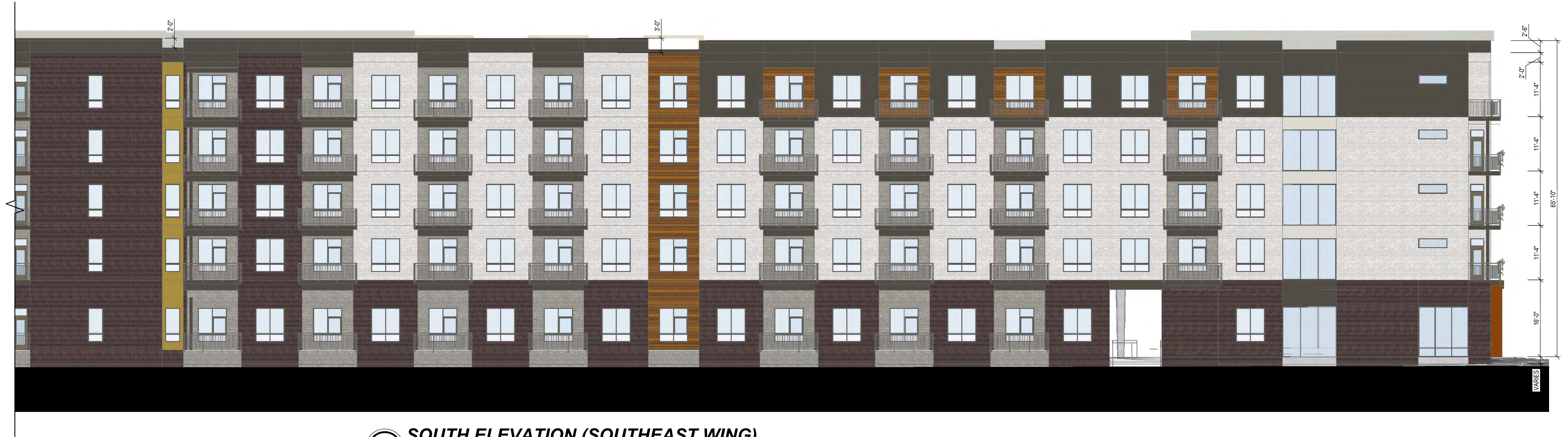
2 SOUTH ELEVATION (SOUTHEAST WING) SCALE: 3/32"=1'-0"
