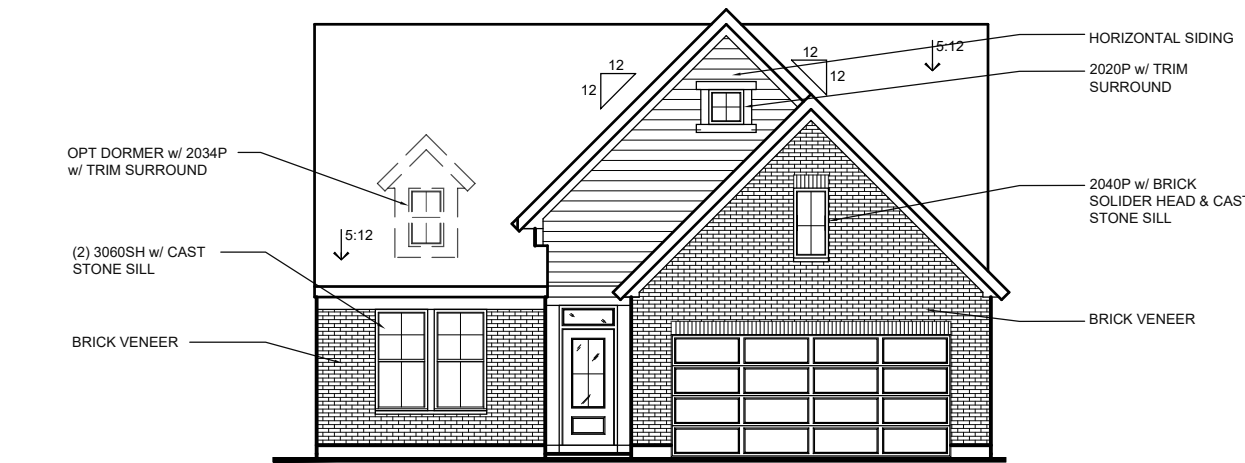
INC. FRONT ENTRY (AVAILABLE w/ LOW OR HIGH BRICK SIDES AND REAR)
