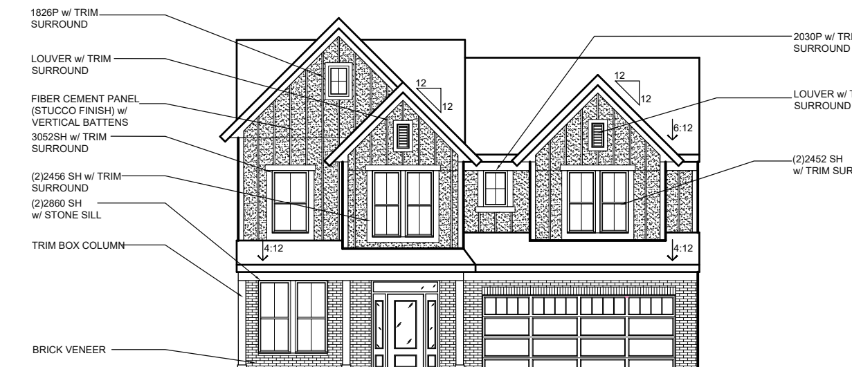
FRONT ENTRY w/ OPT. BRICK VENEER (AVAILABLE w/ LOW OR HIGH BRICK SIDES AND REAR)
