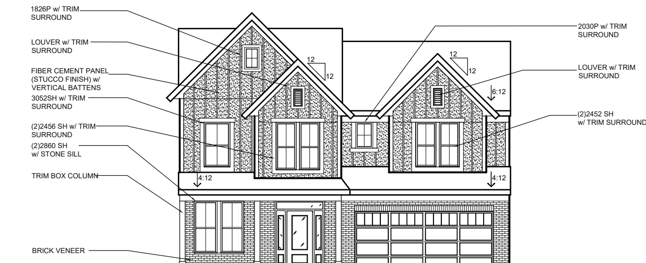
FRONT ENTRY w/ OPT. BRICK VENEER (AVAILABLE w/ LOW OR HIGH BRICK SIDES AND REAR)
