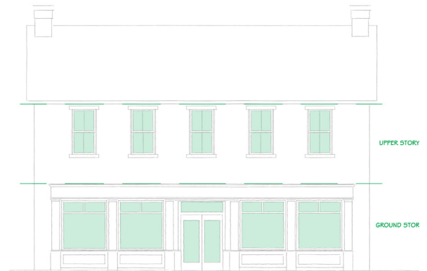
Figure 5.4: Pattern and Proportions of Window/Door Openings.
