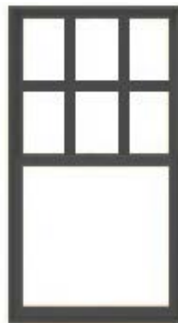
4. Pella Lifestyle Series aluminum clad double-hung window with 6-over-1 traditional simulated-divided-light grille with spacers between glass panes - color Iron Ore (or Andersen or equivalent)
