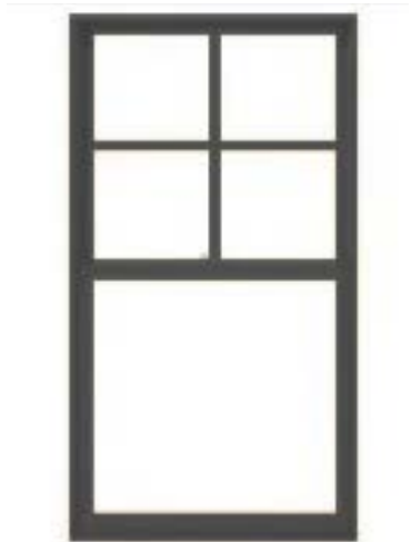
4. Pella Lifestyle Series, aluminum clad double-hung window with traditional simulated-divided-light grille or Andersen or equivalent
