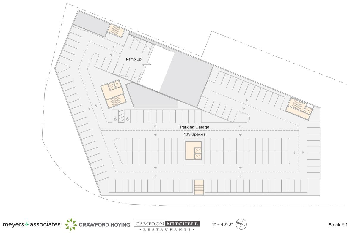
Block Y Mixed Use | Parking Level -3 Floor Plan
