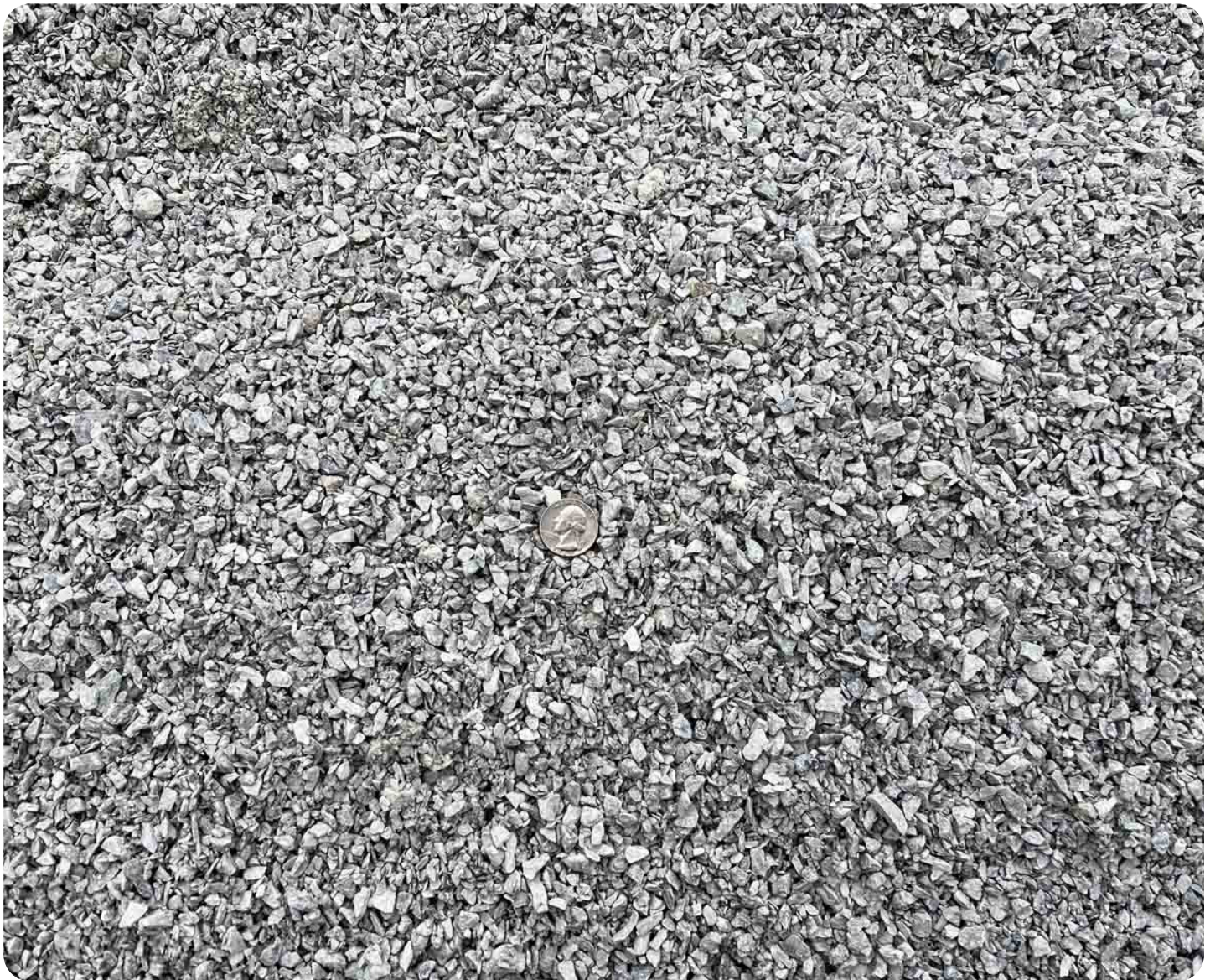
CRUSHED LIMESOTNE FINES 50 / 50 MIX
