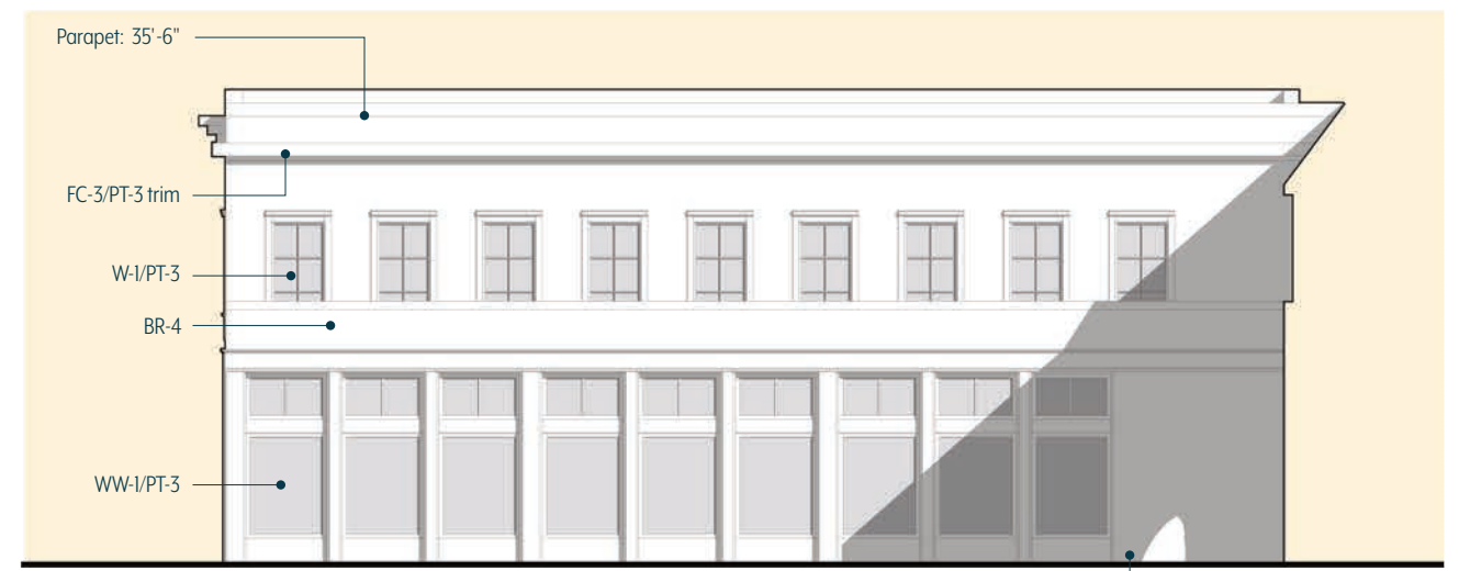
03 BUILDING G - SOUTH ELEVATION Scale: 1/16" = 1' 0 2 4 8
