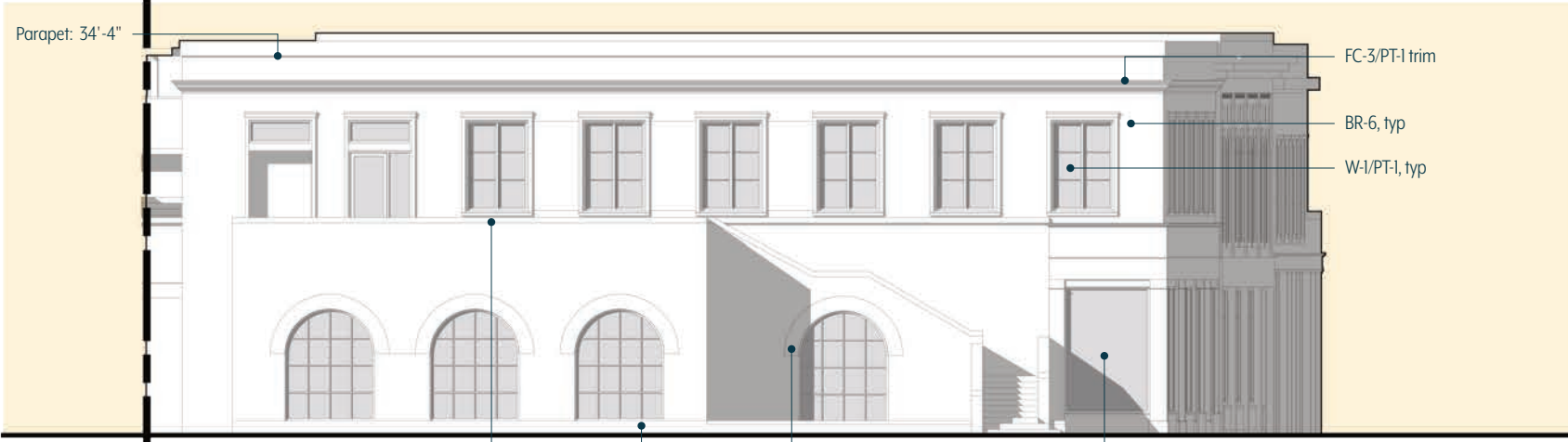
02 BUILDING G - NORTH ELEVATION Scale: 1/16" = 1' 0 2 4 8
