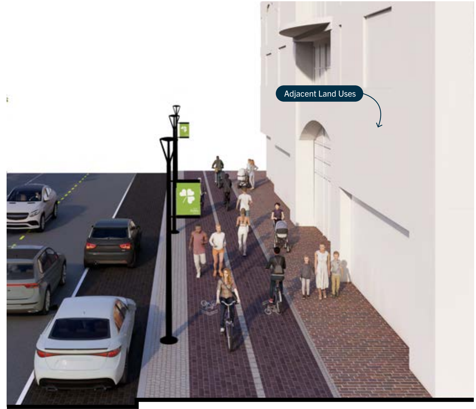
Figure 35. Constrained Urban Trail Section
