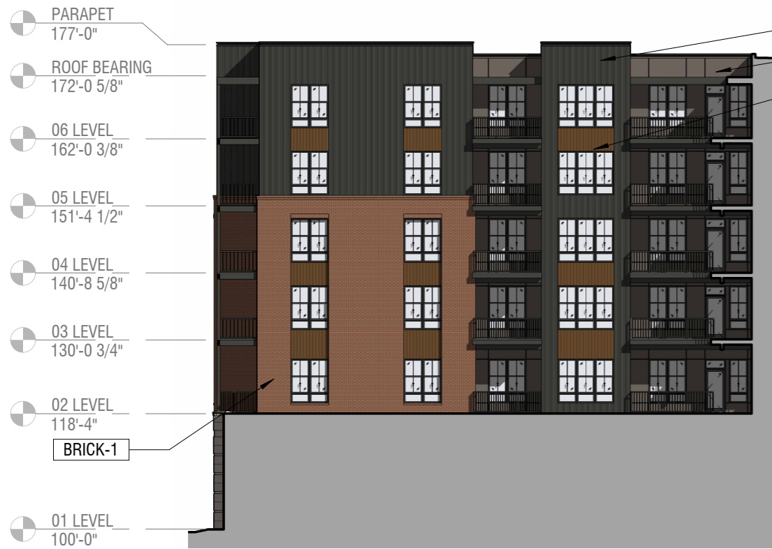
FDP ELEVATION - COURTYARD NORTH SCALE 3/64" = 1'-0"
