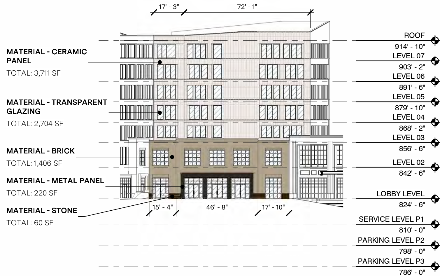
SOUTH BUILDING - NORTH EAST ELEVATION - MATERIALS scale 1/32" = 1'-0"
