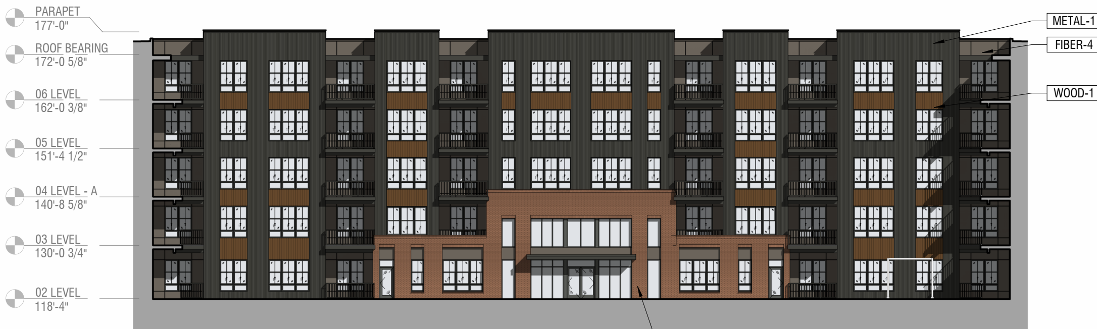
FDP ELEVATION - COURTYARD EAST SCALE 3/64" = 1'-0"
