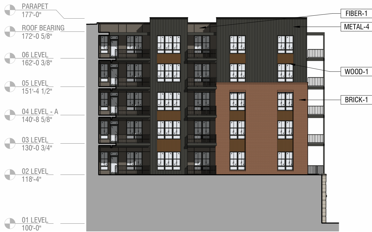
FDP ELEVATION - COURTYARD SOUTH SCALE 3/64" = 1'-0"
