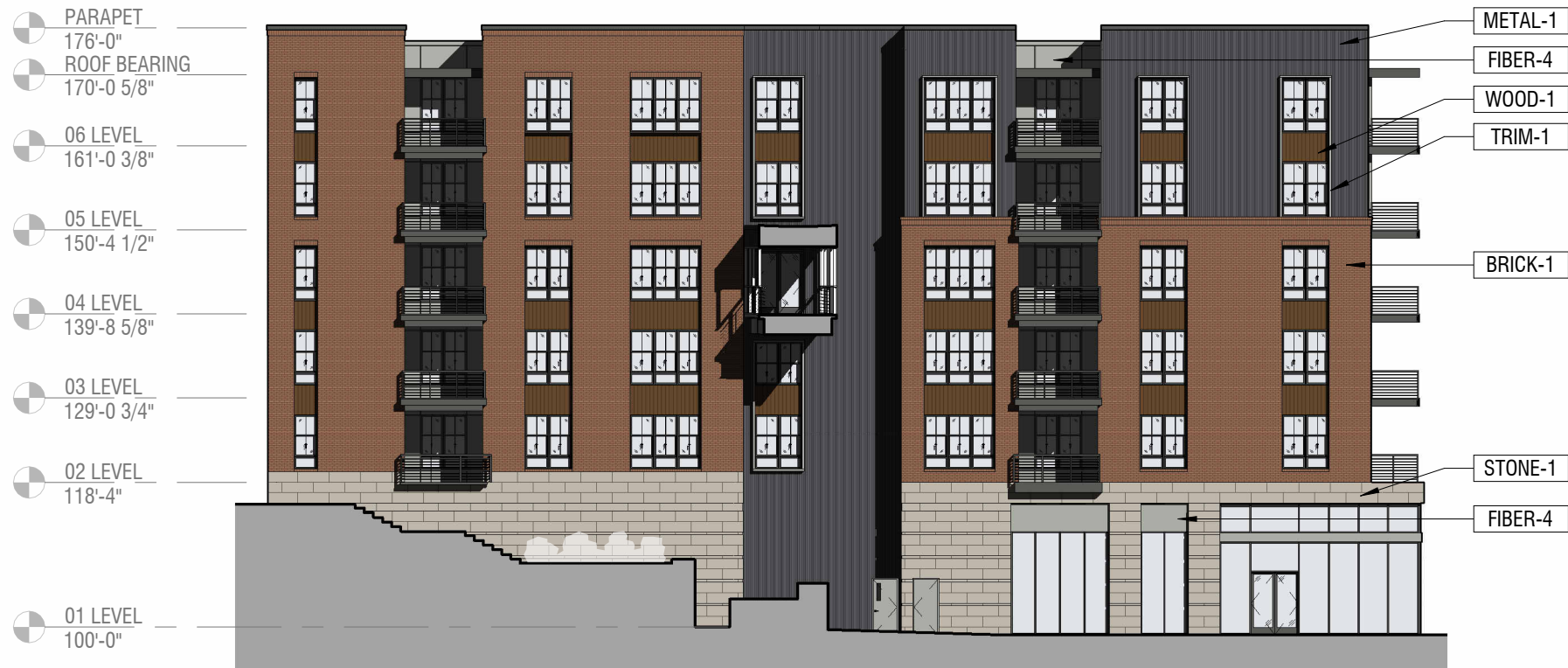
FDP ELEVATION - NORTH SCALE 3/64" = 1'-0"
