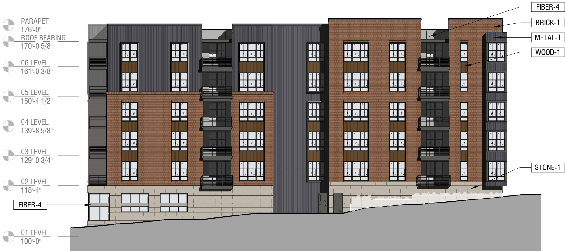
FDP ELEVATION - EAST SCALE 3/64" = 1'-0"
