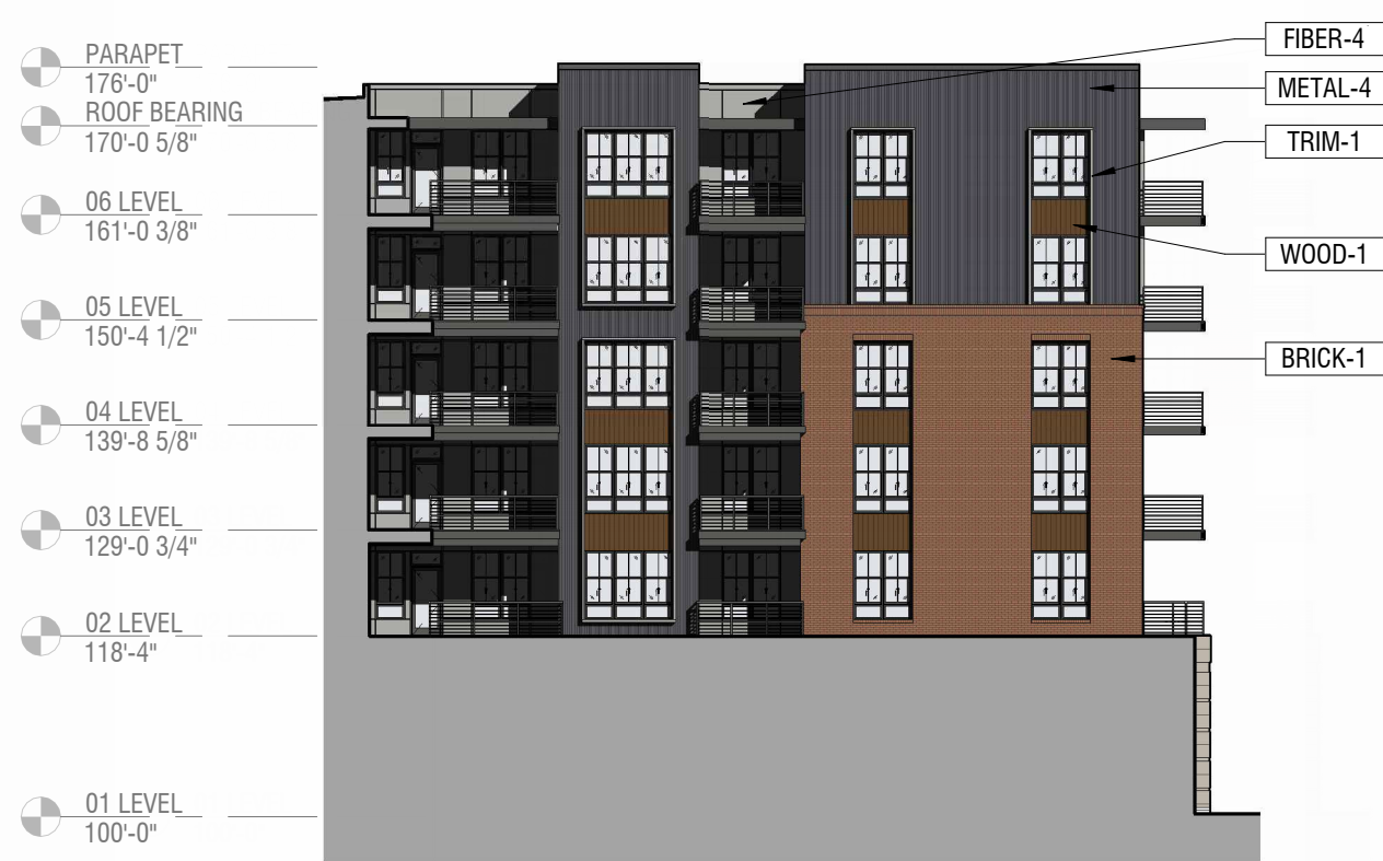
FDP ELEVATION - COURTYARD SOUTH UTH SCALE 3/64" = 1'-0"
