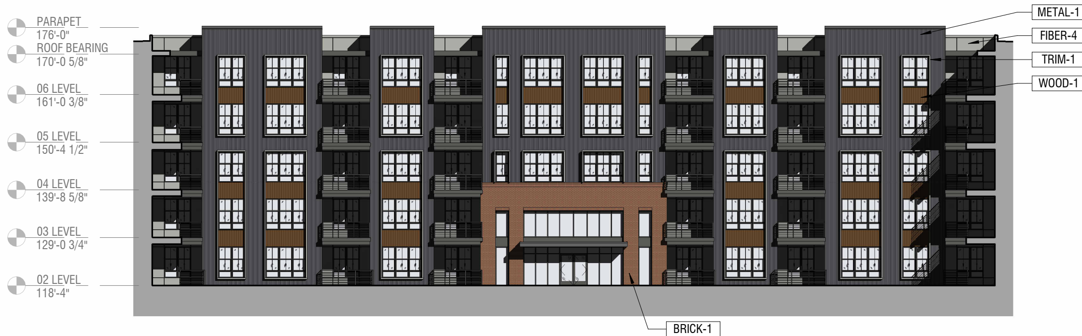
FDP ELEVATION - COURTYARD EAST SCALE 3/64" = 1'-0"
