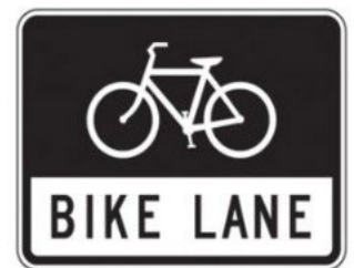
Figure 23. OMUTCD Bicycle Lane Sign R3-17
