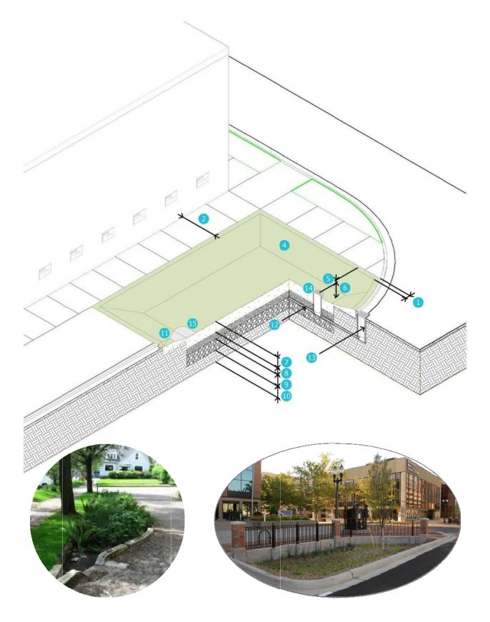
FIGURE 5-9 BIORETENTION CURB EXTENSION DIAGRAM
