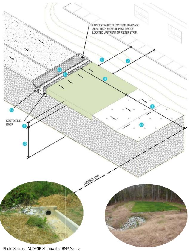
FIGURE 5-3 FILTER STRIP DIAGRAM
