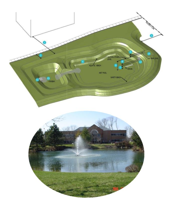
FIGURE 5-13 RETENTION BASIN DIAGRAM
