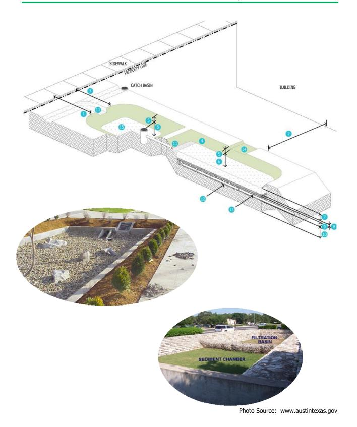
FIGURE 5-4 MEDIA FILTER DIAGRAM
