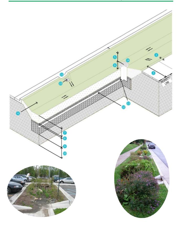
FIGURE 5-6 BIORETENTION SWALE DIAGRAM
