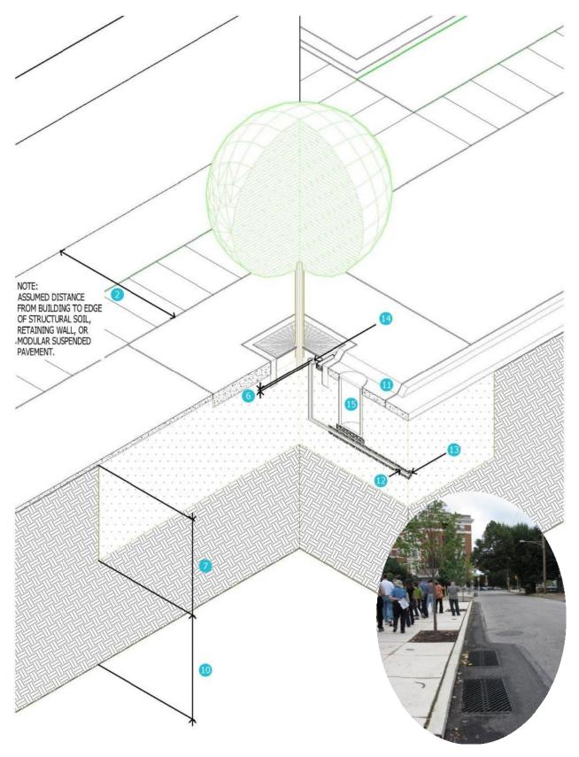
FIGURE 5-8 TREE BOX DIAGRAM
