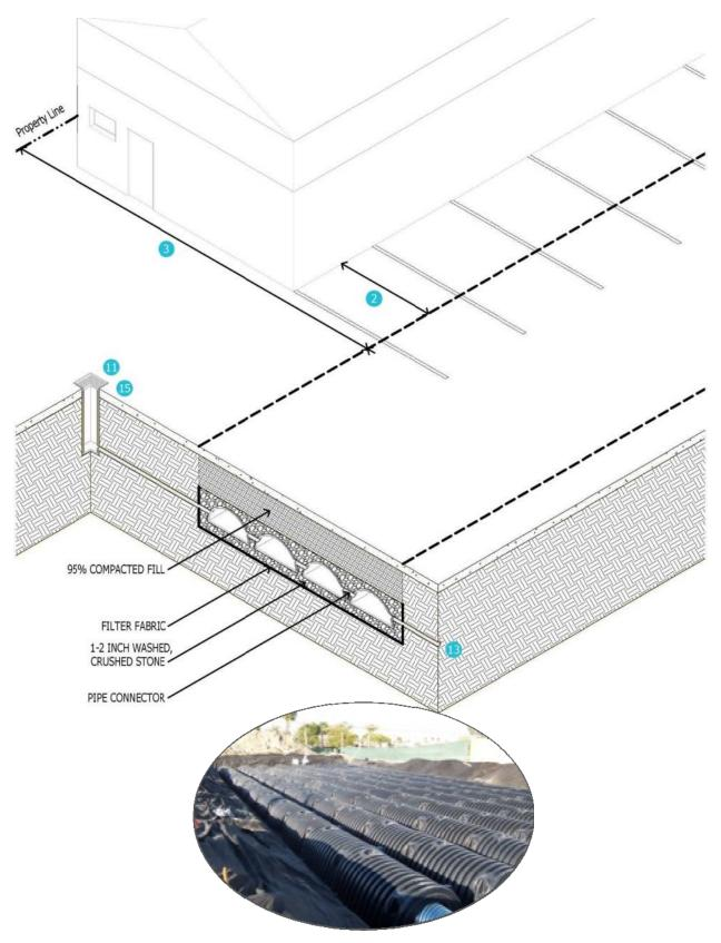
FIGURE 5-16 UNDERGROUND RETENTION/DETENTION
