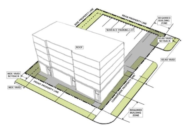
FIGURE 6-3 POTENTIAL ELEMENTS OF A BUILDING SITE
