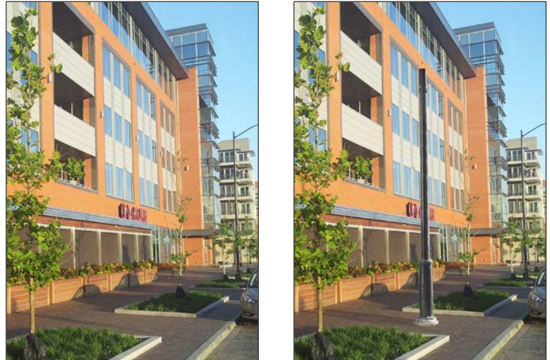
Figure 5.2B--Illustration of Type 2 New Wireless Support Structure Request with Small Cell Equipment within Transformer Base (at right)
