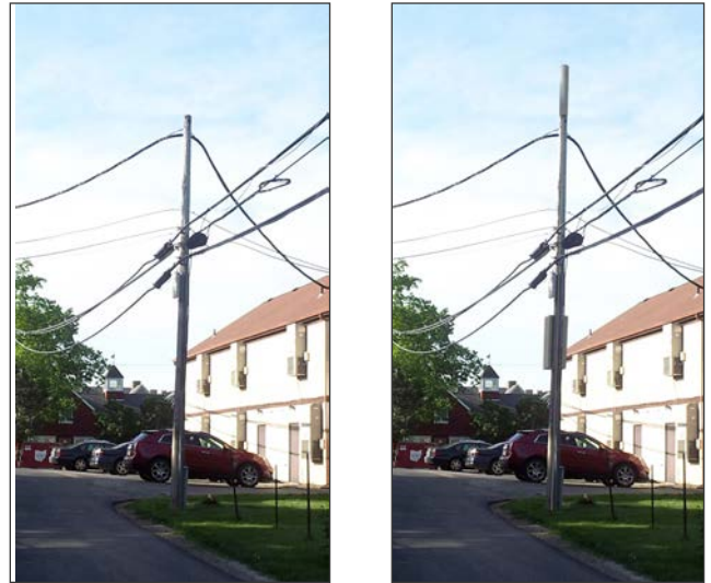
Figure 5.1B--Illustrative Type 1 Collocation Request on Existing Private Wooden Utility Pole (at right)
