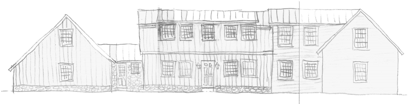
6. Quick sketch of a simplified south elevation. The windows of the second-floor master suite now align with those below and a simplified roofline complements the original structure. The garage addition is reduced in height and its dormers removed so it does not compete with the original building.
