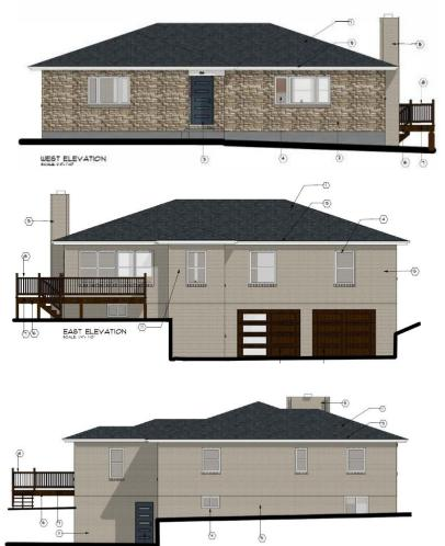
better integrate with the existing rooflines. The stair tower will increase the footprint of the home by approximately 100 square feet. The tower has a pedestrian door on the north elevation, two windows (one on the north and one on the west elevation), and is finished in
