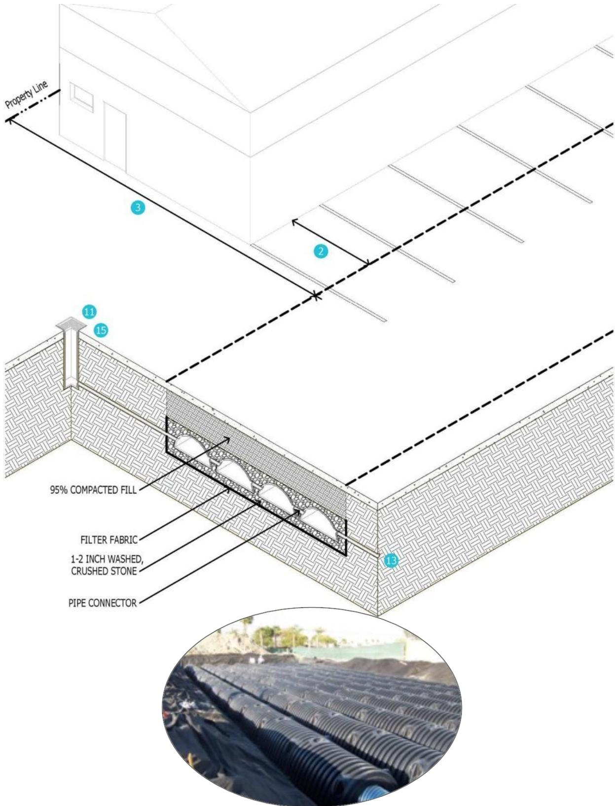
**FIGURE 5-16 UNDERGROUND RETENTION/DETENTION**
