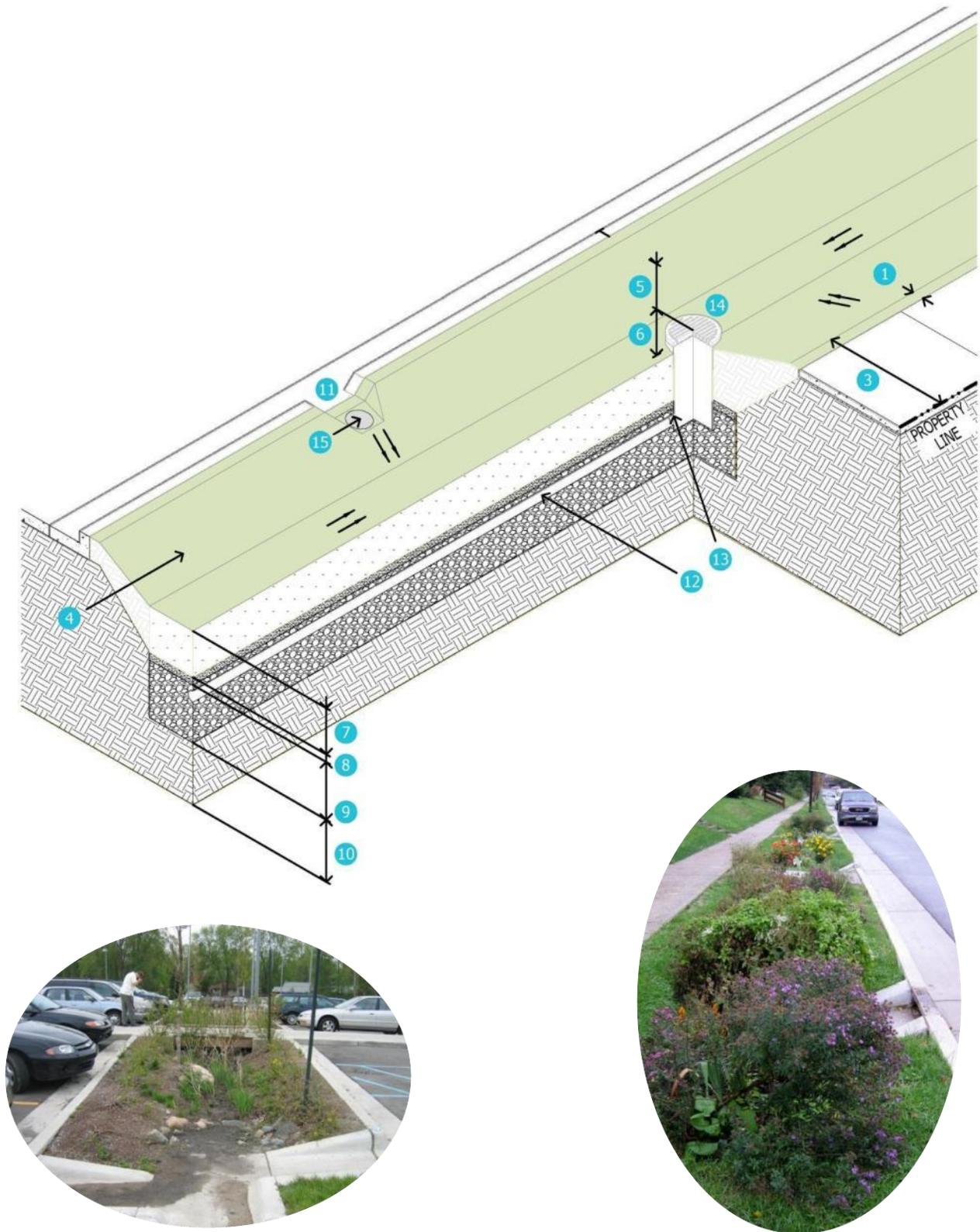
**FIGURE 5-6 BIORETENTION SWALE DIAGRAM**
