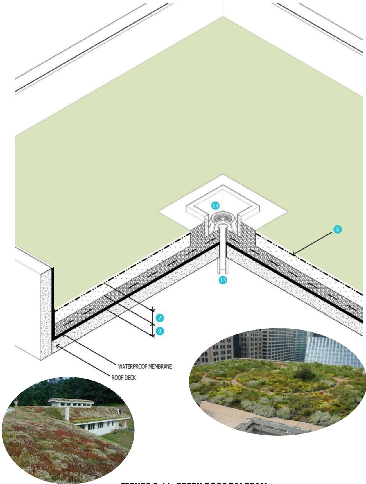
**FIGURE 5-11 GREEN ROOF DIAGRAM**
