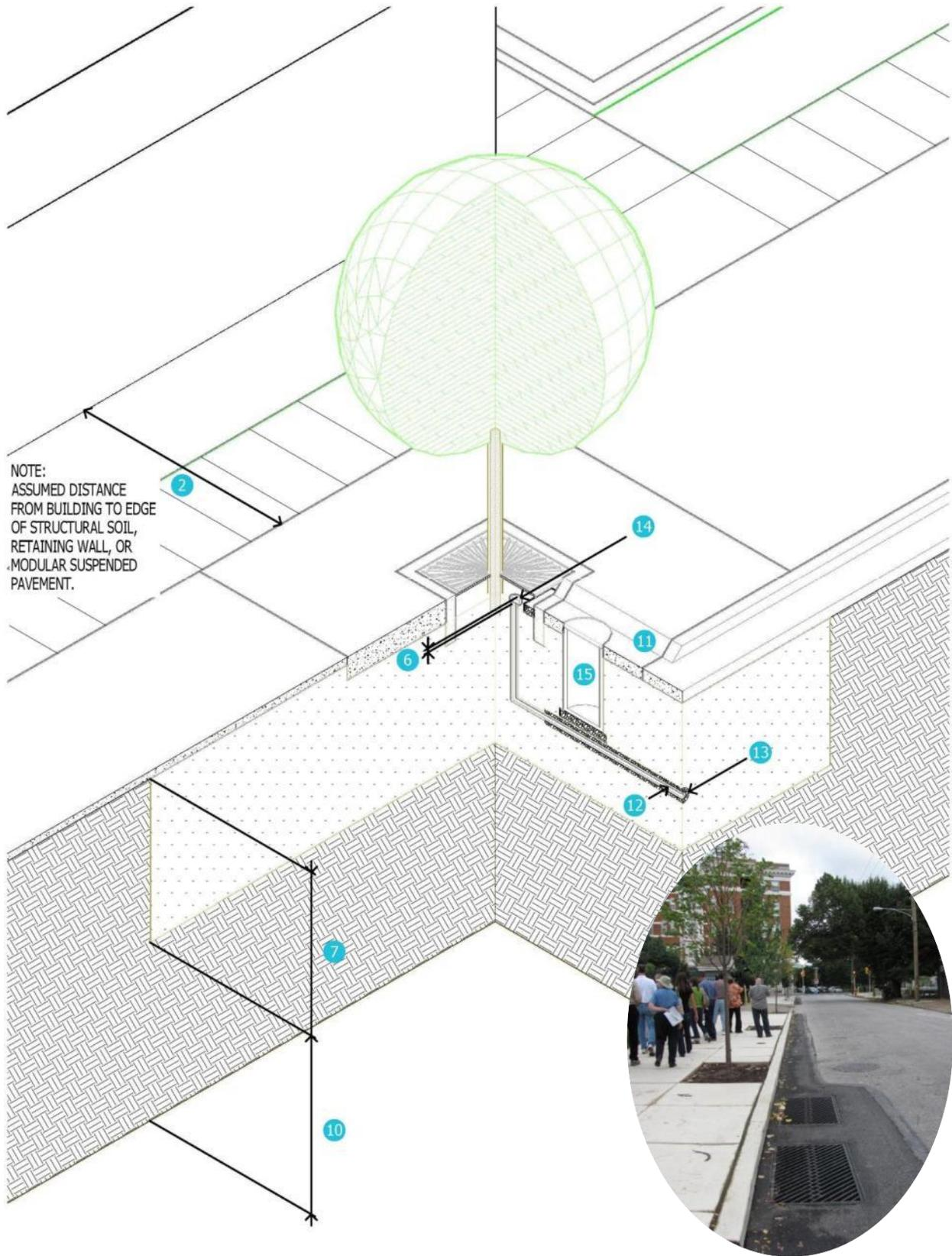
**FIGURE 5-8 TREE BOX DIAGRAM**
