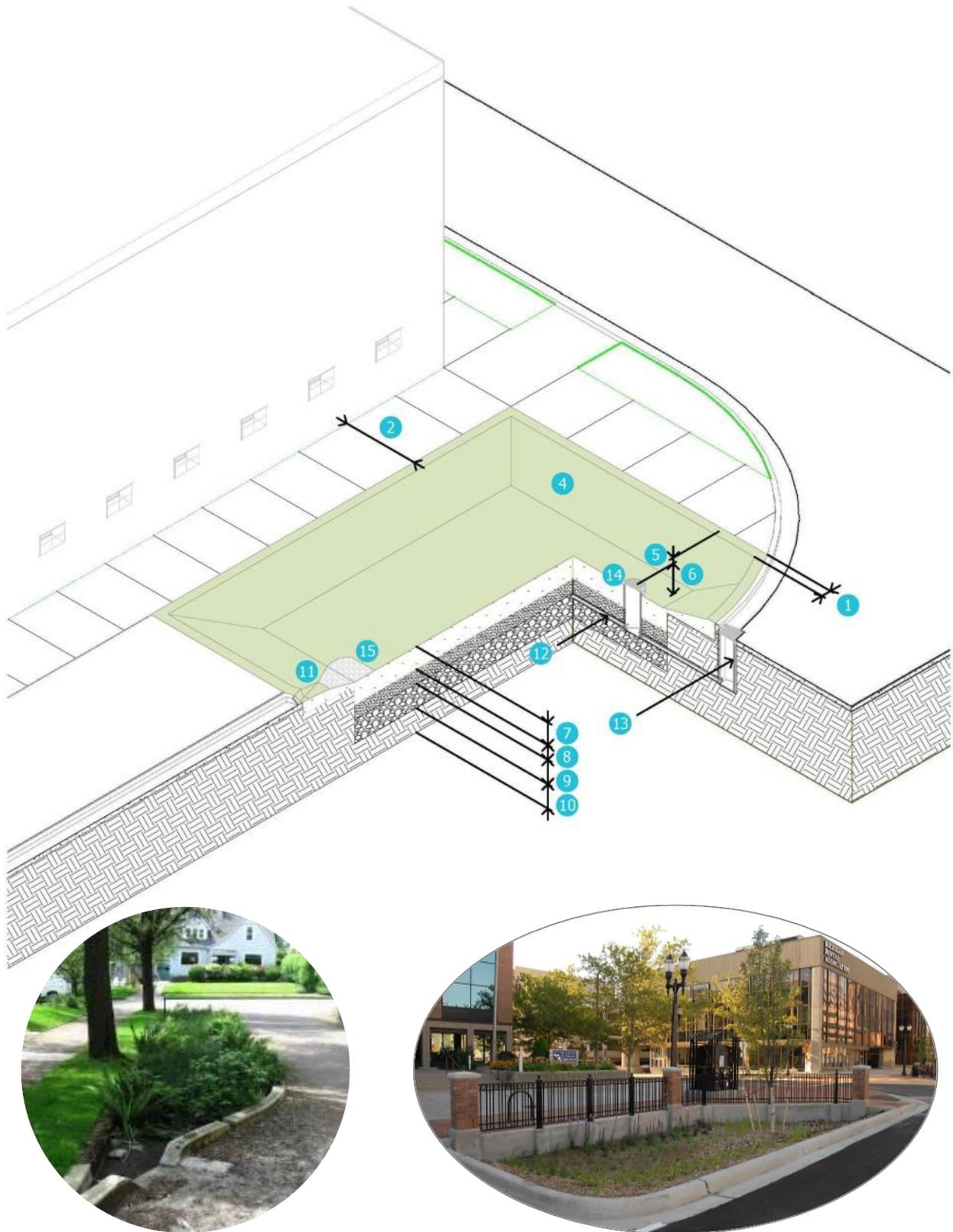
**FIGURE 5-9 BIORETENTION CURB EXTENSION DIAGRAM**
