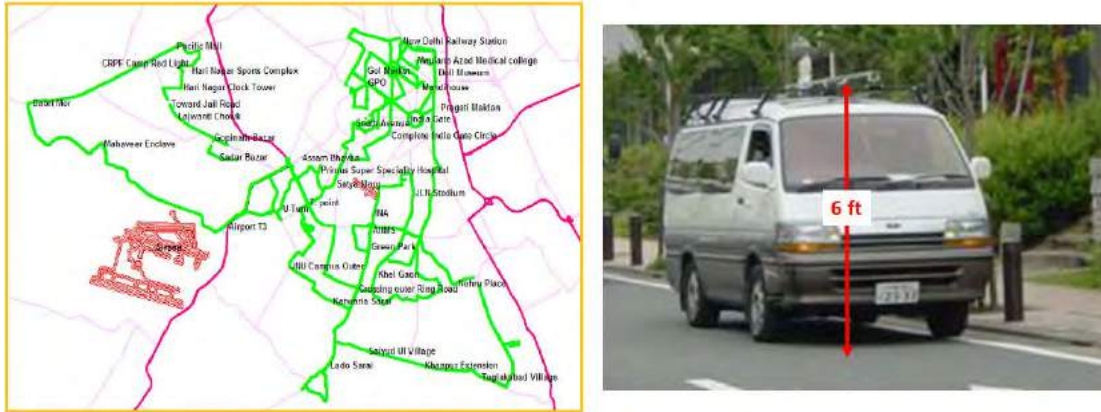
Figure 16 (Left) Drive routes; (right) Rx antenna installed on top of drive test van
