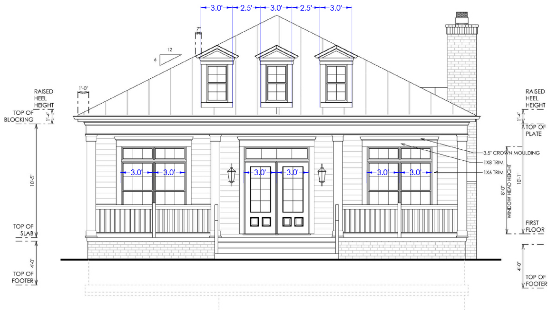
Dormer Width, Spacing and 1 st Floor Rough Opening Widths
