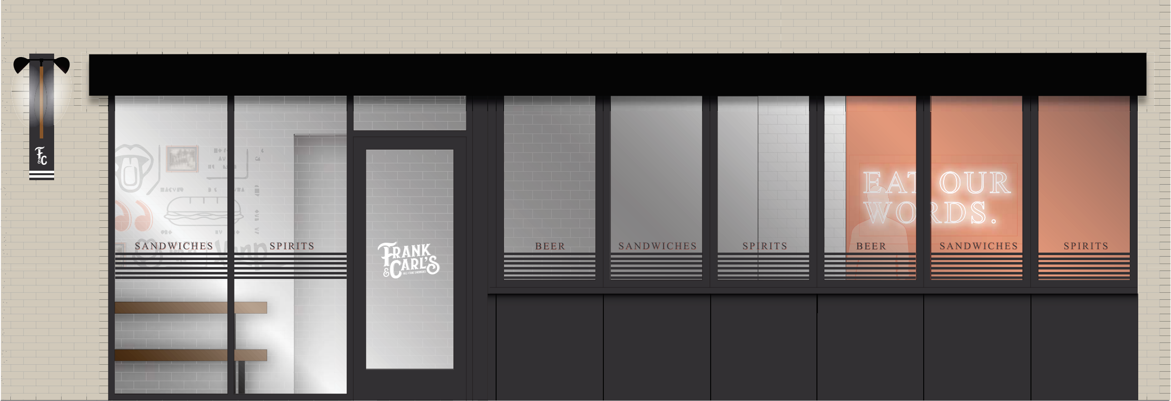
Accordion windows, closed. Black and orange window film words. Black metal paneling under the nano wall, to be same color as window frames.
