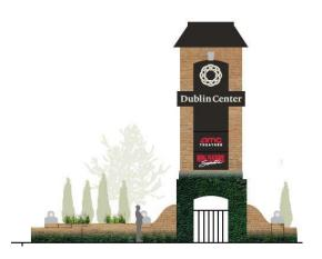
There are four existing signs that are proposed to undergo major refurbishment. Specifically, the clock tower, two large monument entry signs, and one raised monument directional sign. The most significant changes are prosed to the clock tower, which include a new roof, new logo, new name band, new tenant panels, refurbished ironwork, and new landscaping.
