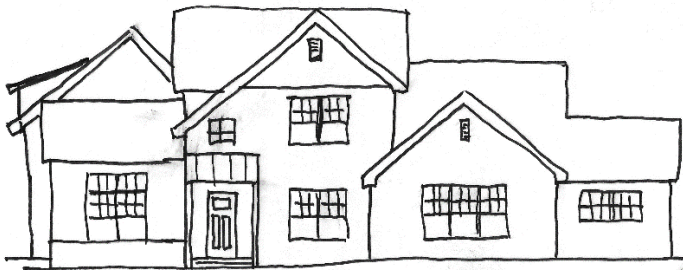
5. Sketch of front elevation with addition located behind the main structure. The front porch and entry have been simplified to complement the saltbox style center bay.
