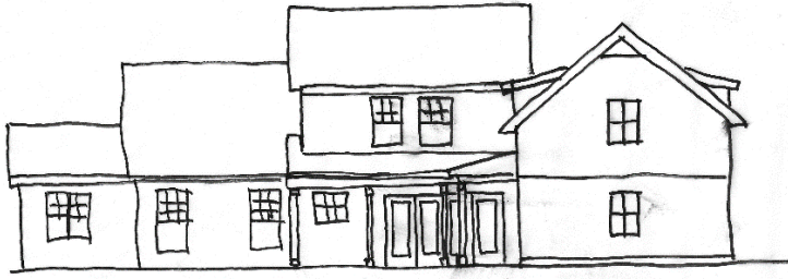
7. Sketch of the rear elevation. The structure of the garage has been simplified so it does not appear so massive. And the front overhang by the garage doors has been removed. The rear porch wraps around to meet that of the main house.
