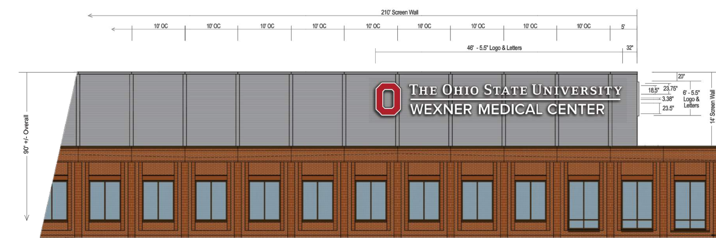
FACE ILLUMINATED WALL GRAPHICS- LOGO GRAPHICS & ADDRESS NUMBERS EAST ELEVATION // Scale 3/32" = 1'
