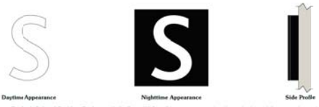
Daytime Appearance | Nighttime Appearance | Side Profile For Dark Colored Building Backgrounds | "SpringHill Suites" letters to appear white during the day and illuminate white at night.
