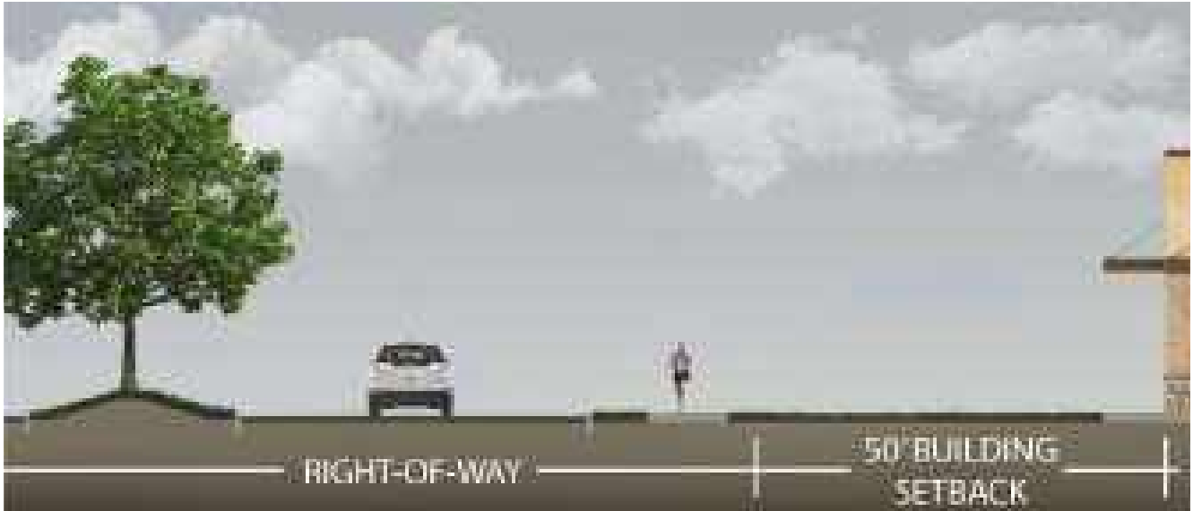
Frantz Road existing condition - typical section
