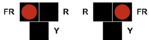
Pedestrian Hybrid Beacon Displaying Alternating Flashing Red During Pedestrian Change Interval
