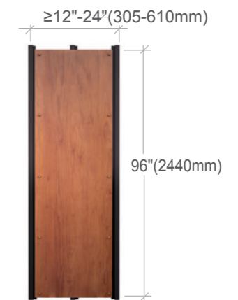
INTERMEDIATE SUPPORT REQUIRED (only 2 rows of fasteners along edge of panel)
