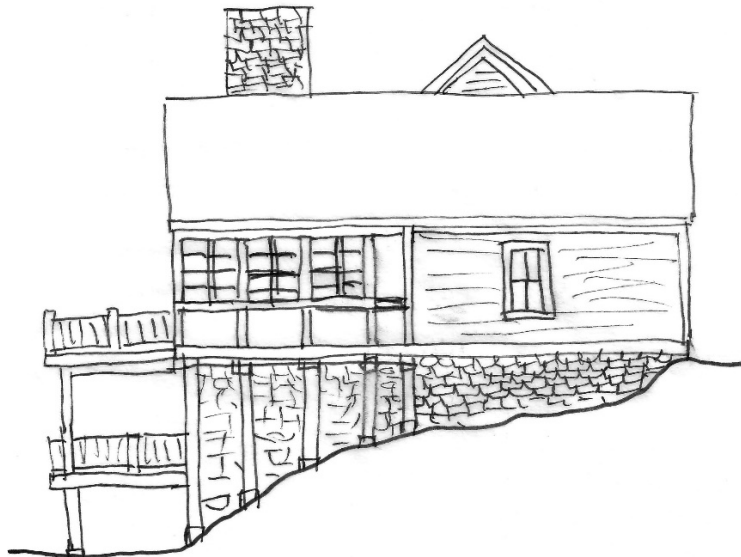
Sketch of revised north elevation with casement windows in sunroom and stone foundation. Note the different material for the sunroom.
