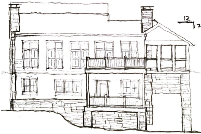
Sketch of rear elevation based on the alternative massing option. (Note the continuous stone foundation on the “original” house and garage and a lowered stone foundation on the “addition.”) Elsewhere is horizontal siding. The “addition’s” window should be the same type as on the “original” house (double-sashed), and both chimneys should have more simple caps. Note that the open porch’s chimney continues to the ground.
