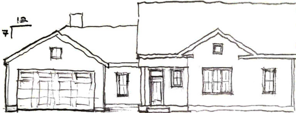
Sketch of revised west elevation with the “original” house on the right, its garage on the left, and the connector between them. This sketch uses an alternative massing design to consider. Sash windows are traditional to the area; consider changing the window type to double-hung. Note the simplified detailing around the windows and the entry porch.
