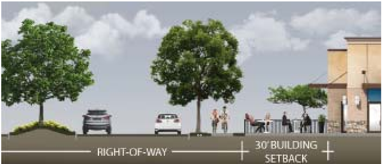
Frantz Road proposed condition - typical section
