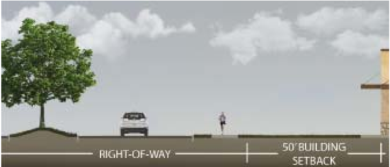
Frantz Road existing condition - typical section
