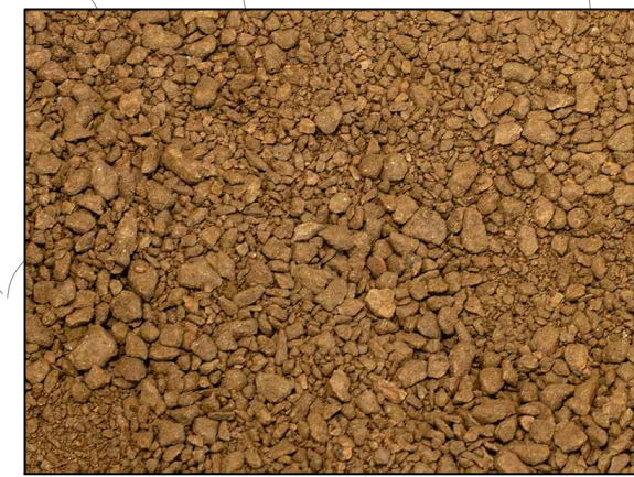
decomposed granite (honey) (beige, natural product, 3/4" down to fines, obtained from Semco Outdoor)
