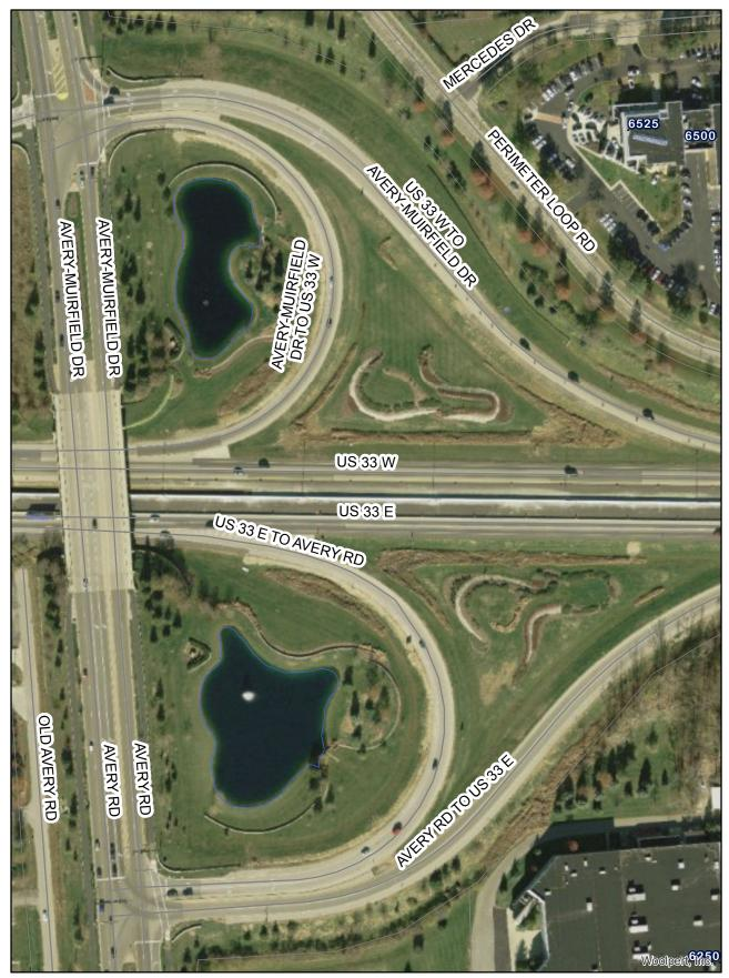
North Pond Surface Acres: 0.62 Average Depth: 7.66 Acre Feet: 4.74 (used for irrigation) South Pond Surface Acres: 0.88 Average Depth: 9.69 Acre Feet: 8.48 (used for irrigation)
