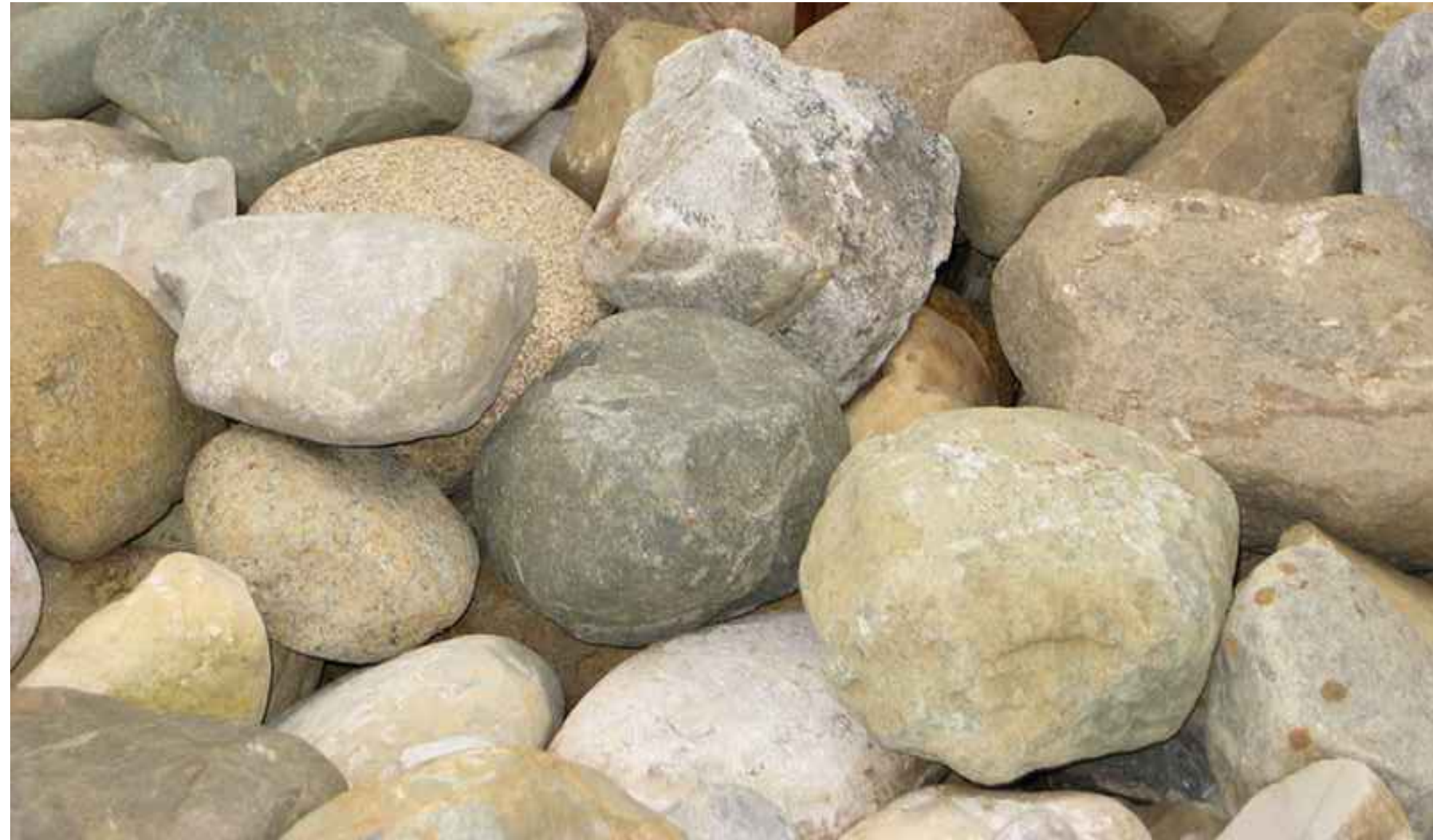
DECORATIVE RIP RAP SHALL BE CLEAN WASHED, ROUNDED RIVER STONE 3"-6". BASIS OF DESIGN LANG STONE DARBY.
