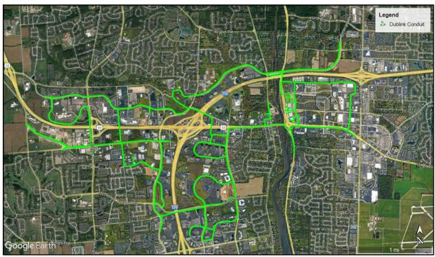
The green line is the existing Dublink conduit system with available capacity.
