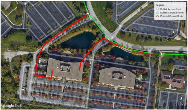
The green line is an existing Dublink conduit with available capacity. Red lines are potential lateral conduit routes to connect to existing conduits inside 565 Metro Place that will connect up to Dart Points Data Center MMR and/or Data Center space.
