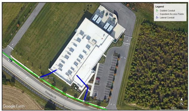
The green line is an existing Dublink conduit with available capacity. The blue line is the existing Expedient lateral conduit to get into the MMR and/or Data Center space.
