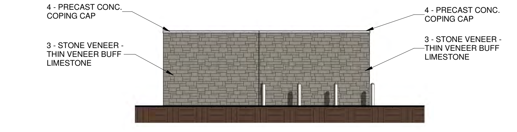
7 GEN/TRASH ENCLOSURE NORTH ELEVATION 1/8" = 1'-0"
